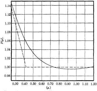
Fig. 1.—The correction factor  $F(\rho)$  giving the dependency of interionic distance in sodium chloride type crystals on the radius ratio  $\rho$ (solid line). The broken line shows the form of this function for  $n = \infty$ ; that is, for solid spheres.
